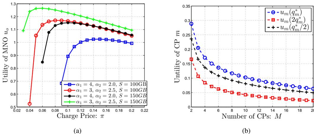
Figure 2: Numerical results for the proposed Stackelberg game with (a) utility function of the MNO with respect to charge price  $\pi$  for 2-CP case, and (b) utility of the CP with respect to the total number of CPs  $M$  under different caching requests.
