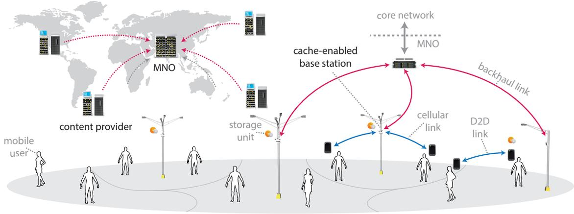
Figure 1: An example of caching scenario where multiple CPs are competing for caching their contents at the cache-enabled base stations of the MNO, therefore satisfying their users in that geographical region.
