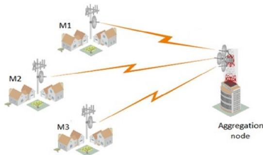
Figure 1: Backhaul network. The aggregation node handles all the traffic produced by and to nodes M1, M2, M3.
