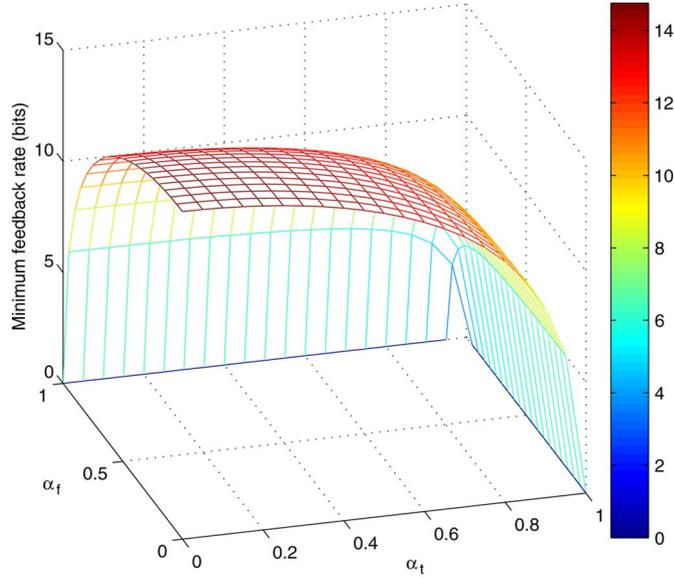
Fig. 3. Minimal differential feedback rate for  $N_r = 2$ ,  $N_t = 2$ ,  $\sigma_H^2 = 1$ , and  $D = 0.1$ .
