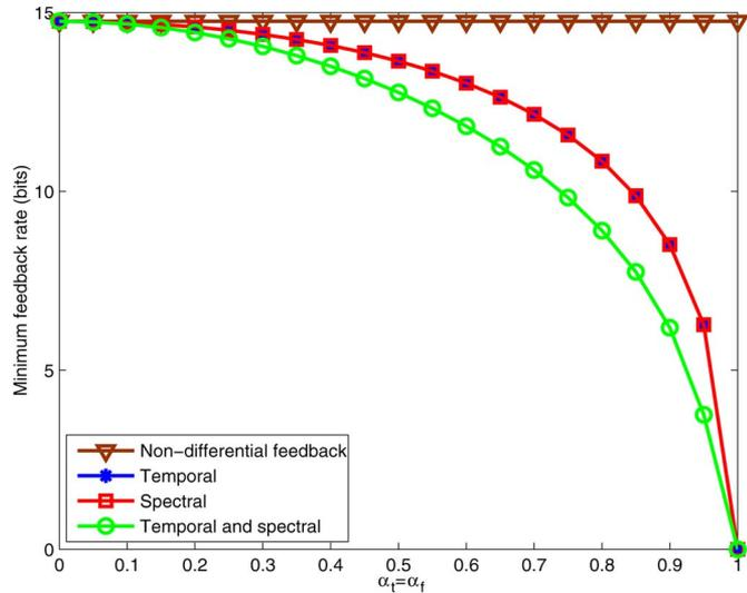
Fig. 4. Relationship between the minimal feedback rate and temporal and spectral correlations, when they are equal, for  $N_r = 2$ ,  $N_t = 2$ ,  $\sigma_H^2 = 1$ , and  $D = 0.1$ .
