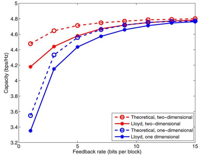
Fig. 5. Relationship between the ergodic capacity and the feedback rate with Lloyd's algorithm in AR1 model for  $N_r = 2$ ,  $N_t = 2$ ,  $\sigma_H^2 = 1$ , and SNR = 5 dB.
