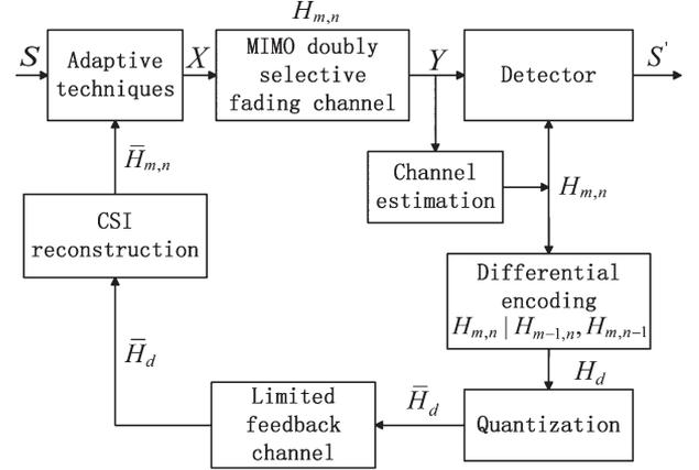
Fig. 1. System model of the differential feedback over MIMO doubly selective fading channels.
