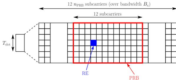
Fig. 1. Time-frequency resource grid in an LTE downlink slot.
