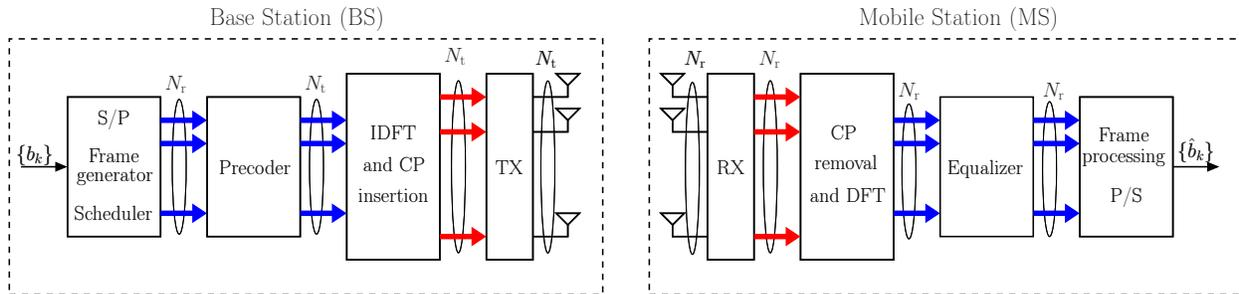
Fig. 2. System model for the considered OFDM MU-MIMO downlink system. Thicker lines correspond to vectors of OFDM symbols for each antenna, with size  $N_c$  (blue lines) or  $N_c + N_g$  (red lines).
