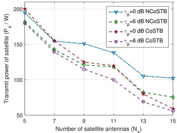
Fig. 5. Transmit power of the satellite versus the number of antennas carried on the satellite  $N_s$  and BSs' SINR threshold  $\gamma_p$ .
