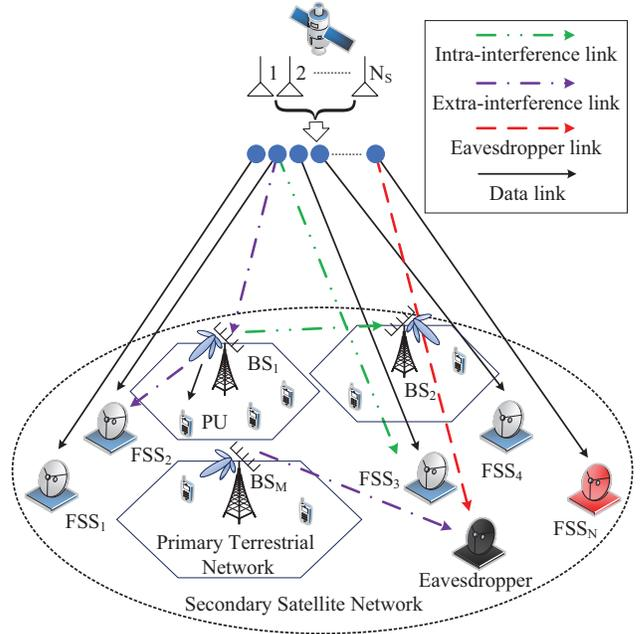
Fig. 1. The coexistence system of SatCom and terrestrial cellular networks.
