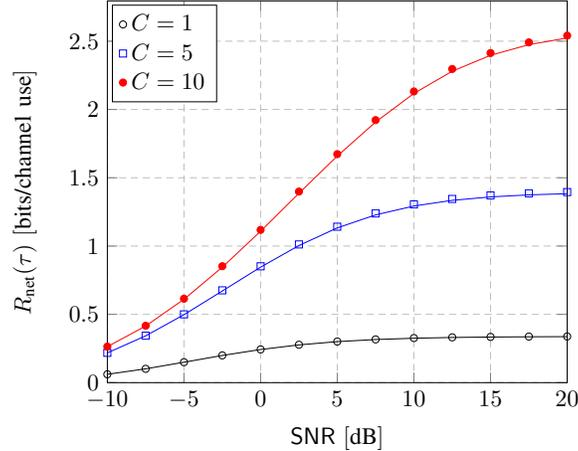
Fig. 3. Net ergodic achievable rate  $R_{\text{net}}(\tau)$  vs SNR for  $\tau = 40$  and  $T = 1000$ . The markers are obtained by simulations, the solid lines correspond to the deterministic equivalent  $\bar{R}_{\text{net}}(\tau)$ .
