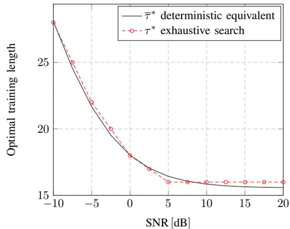
Fig. 5. Optimal training length  $\tau^*$  and  $\bar{\tau}^*$  vs SNR for  $C = 1$  bits/channel use and  $T = 100$ . The solid line corresponds to  $\bar{\tau}^*$  maximizing  $\bar{R}_{\text{net}}(\tau)$ , the dashed line corresponds to  $\tau^*$  maximizing  $R_{\text{net}}(\tau)$  and is obtained by an exhaustive search based on Monte Carlo simulations.
