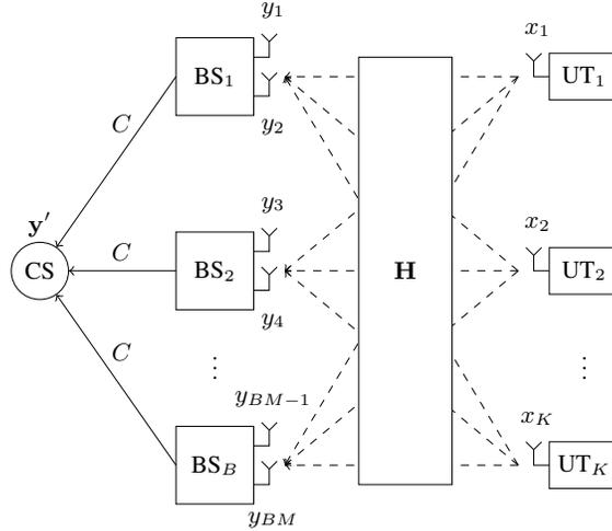
Fig. 1. Schematic system model for  $M = 2$  antennas per BS. The BSs compress and forward their received signals to the CS via orthogonal backhaul links of capacity  $C$  bits/channel use. The CS jointly processes the received data from all BSs.
