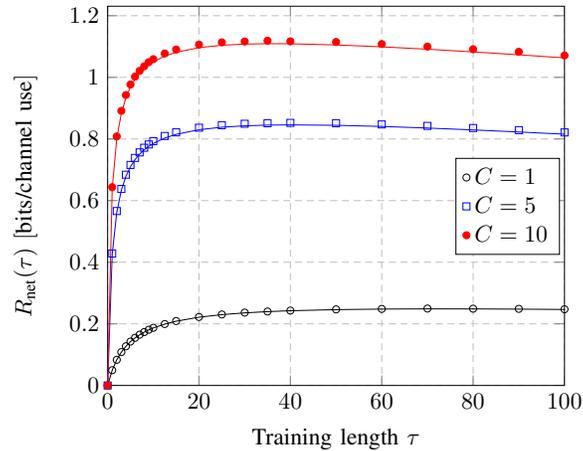
Fig. 4. Net ergodic achievable rate  $R_{\text{net}}(\tau)$  vs training length  $\tau$  for SNR = 0 dB and  $T = 1000$ . The markers are obtained by simulations, the solid lines correspond to the deterministic equivalent  $\bar{R}_{\text{net}}(\tau)$ .
