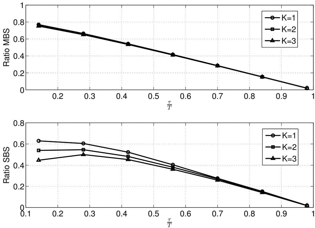
Figure 9. Ratio between the rate obtained with imperfect CSIT and the rate obtained with perfect CSIT for macro cell and small cell system as  $K$  changes, and  $\beta = 1$  ( $N = 24$ ,  $L = 6$  and bandwidth of 0.48 Mhz).
