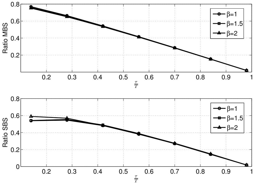
Figure 8. Ratio between the rate obtained with imperfect CSIT and the rate obtained with perfect CSIT for macro cell and small cell system as  $\beta$  changes, and  $K = 3$  ( $N = 24$ ,  $L = 6$  and bandwidth of 0.48 Mhz).
