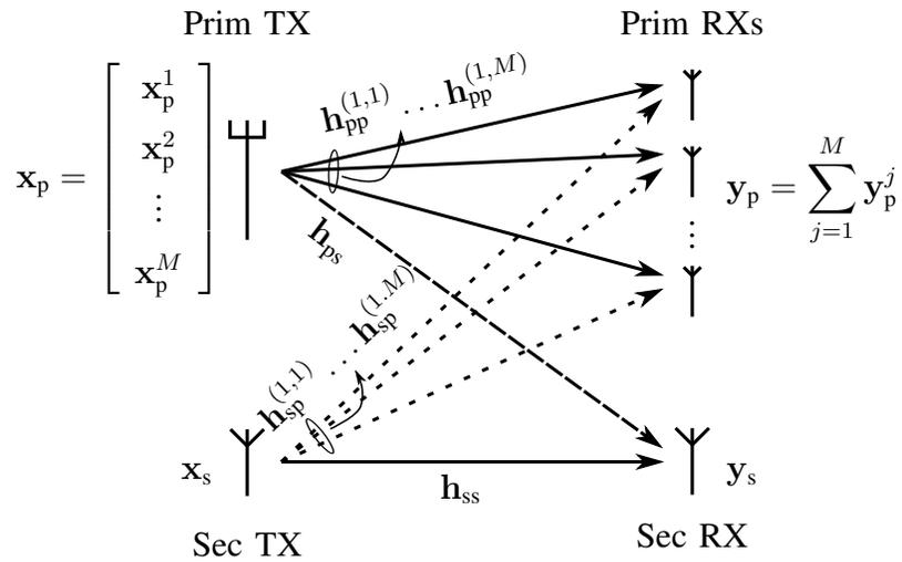
Figure 2. OFDMA downlink interference channel model, single SBS
