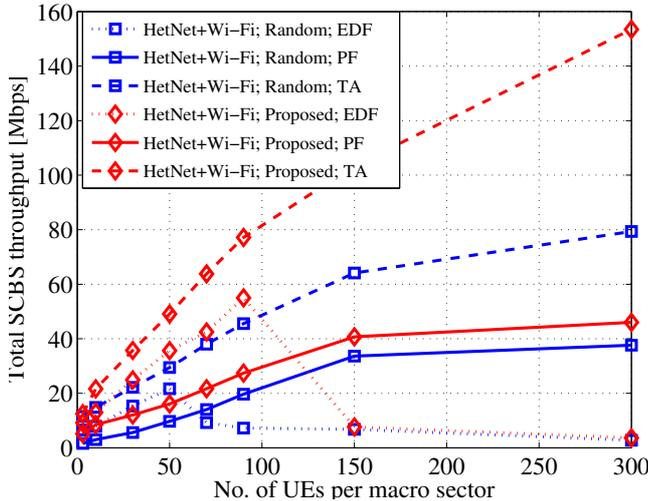
Fig. 5. Total cell throughput vs. number of users.
